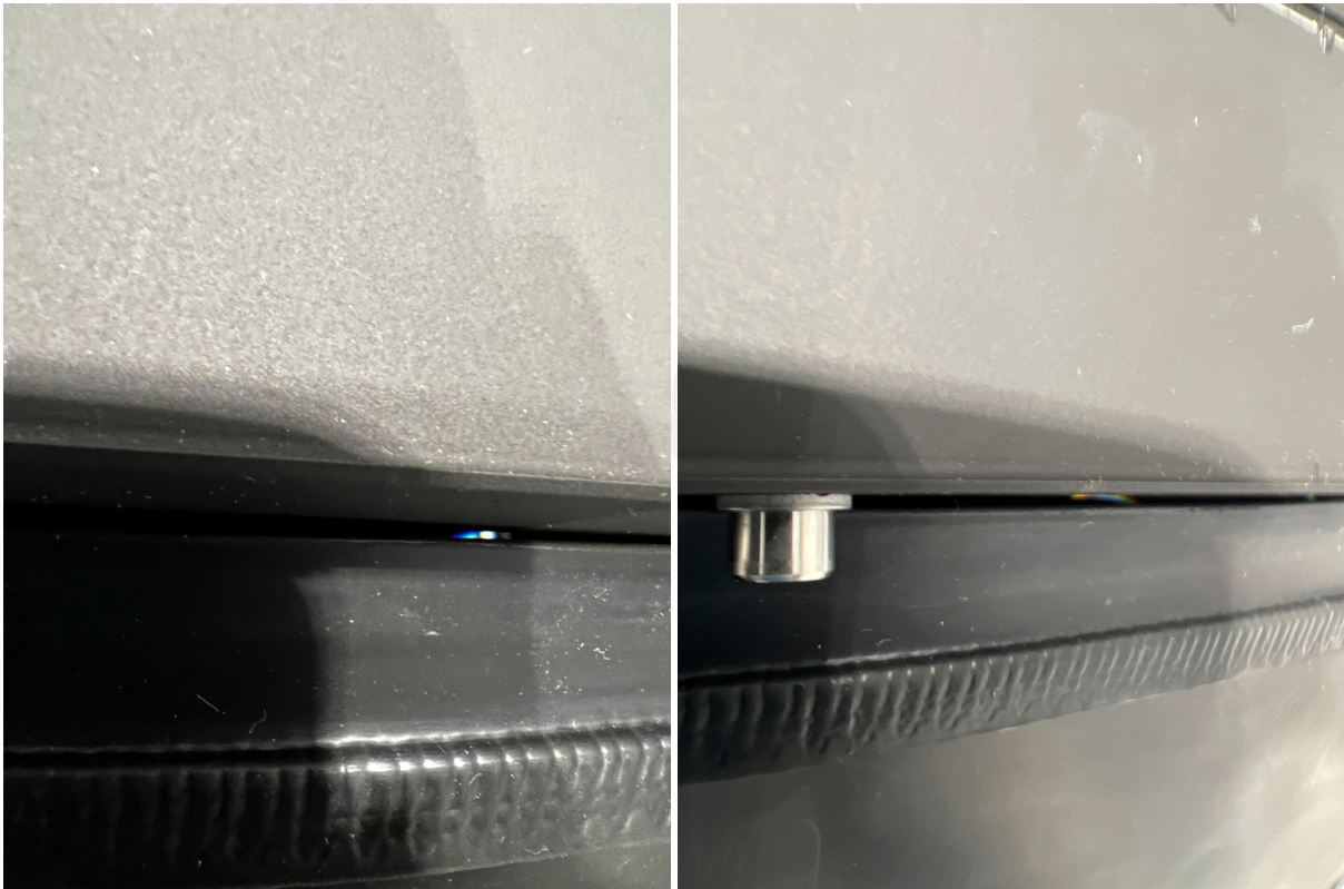
Figure 10: Example photos of the L1 cover gaps. These were covered by tape where we could safely apply it and by the black shroud.
