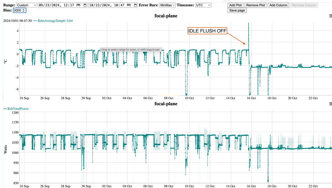
Figure 28: Impact of enabling and disabling IDLE_FLUSH on focal-plane temperature and power consumption.
