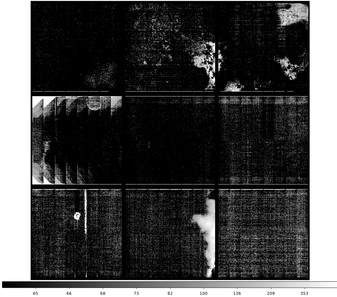
Figure 49: Phosphorescence transients for the R01 RTM captured in the first 15 s following red CCOB LED at 400 ke/pix. With 8»8 blocking, the upper end of the color scale (640) corresponds to 10 e/pixel when averaged over 64 pixels contributing.
