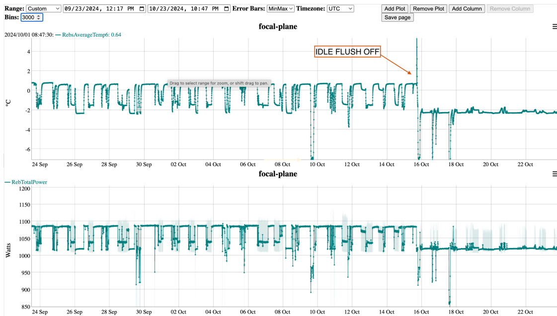
Figure 27: Impact of enabling and disabling IDLE_FLUSH on focal-plane temperature and power consumption.
